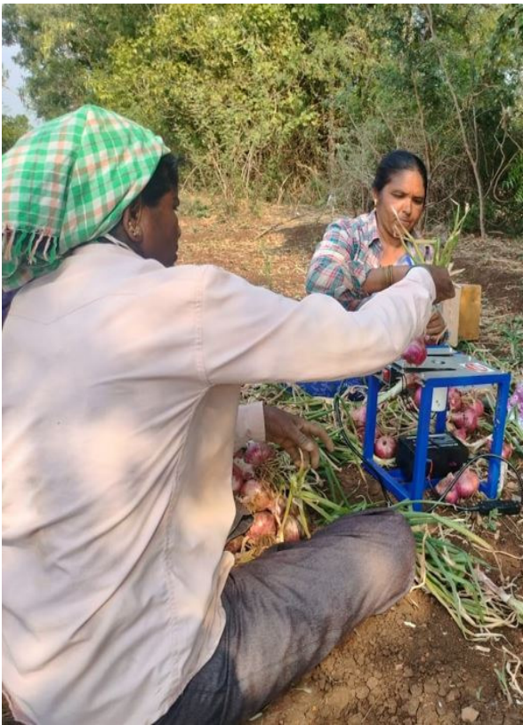
Fig. 2 : Two persons handling the onion detopper simultaneously
